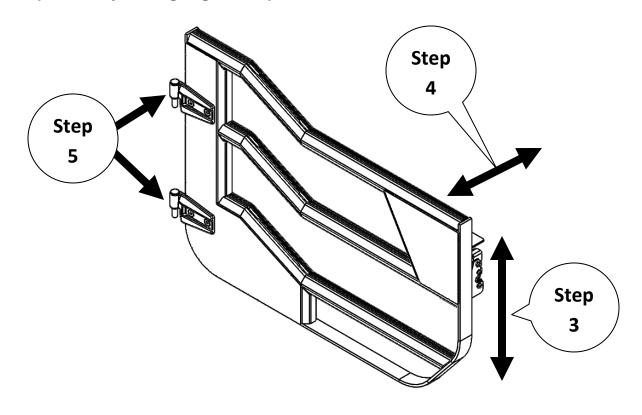
To adjust doors up and down use a 4mm Allen wrench and a 10mm wrench to loosen the 3 bolts and move latch up or down. Once adjusted, fully tighten hardware.
