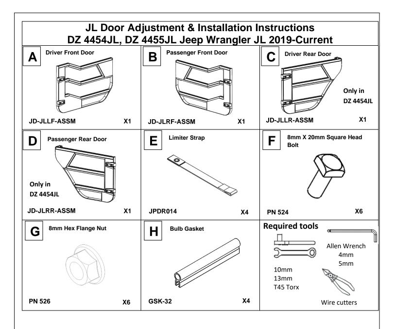
First Install the gasket (H) on the door frame between the top and middle bar. Press firmly to ensure the gasket is fully installed.
