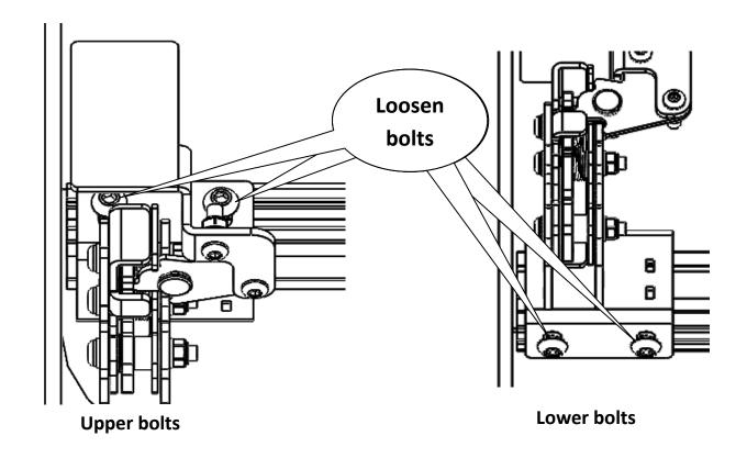
To adjust hinges use a T45 Torx and a 13mm wrench. Once adjusted, fully tighten hardware.
